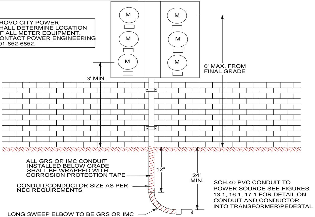
Figure 7.1 Multi-meter Installation
