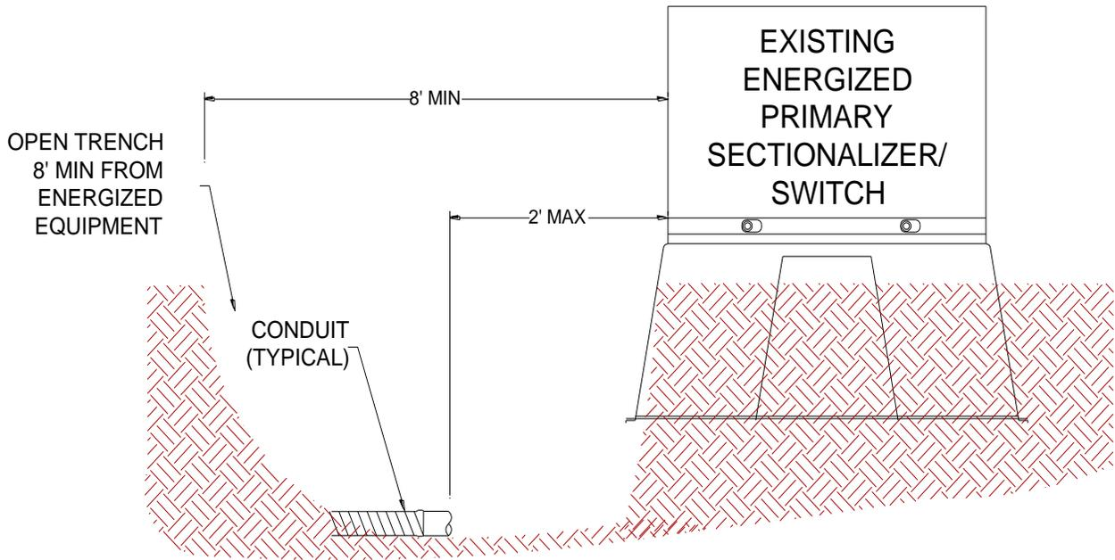
Figure 15.1.1 Connecting to a Sectionalizer
