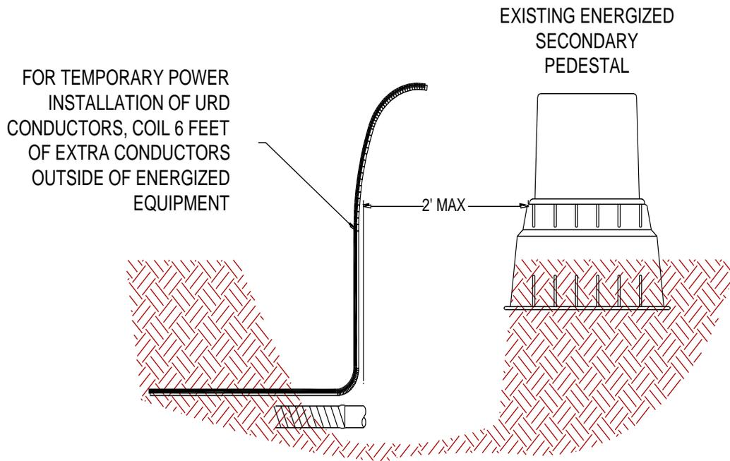
Figure 15.1.2 Connecting to a Pedestal
