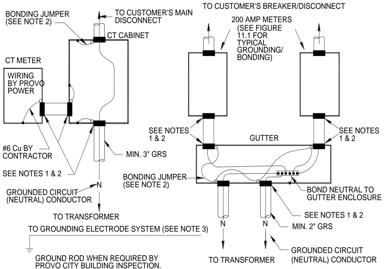
Figure 19.1 Typical CT Cabinet Grounding and Bonding
