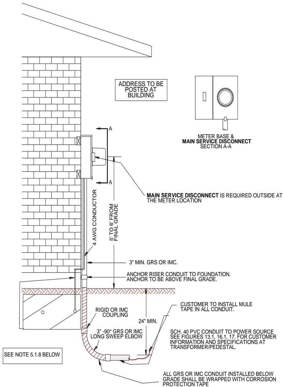
Figure 5.1 Underground Service Installation
