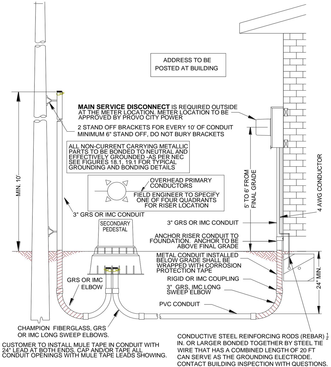
Figure 8.1 OH to U.G. Service Installation
