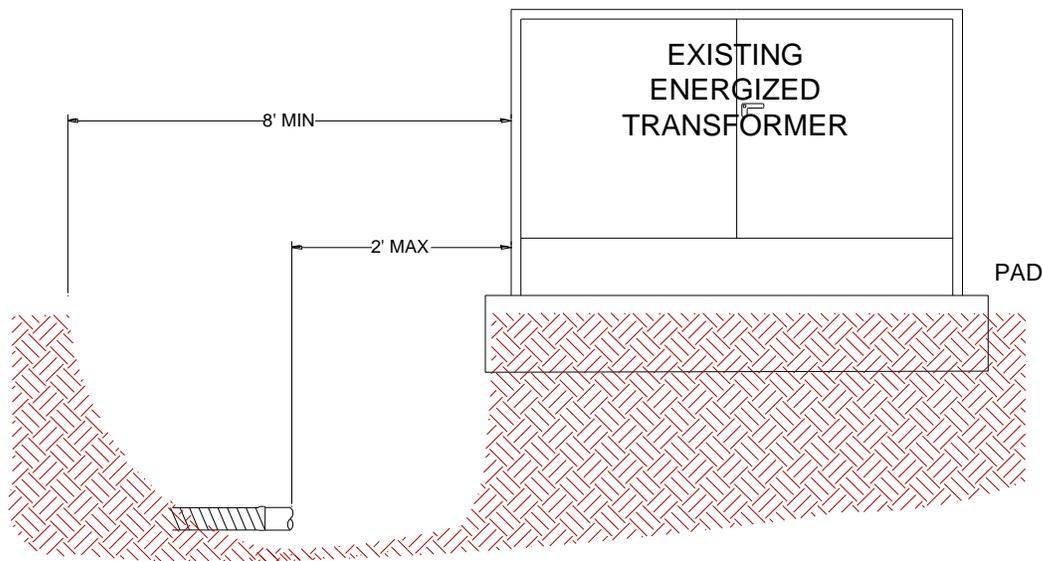
Figure 15.1.3 Connecting to a Transformer
