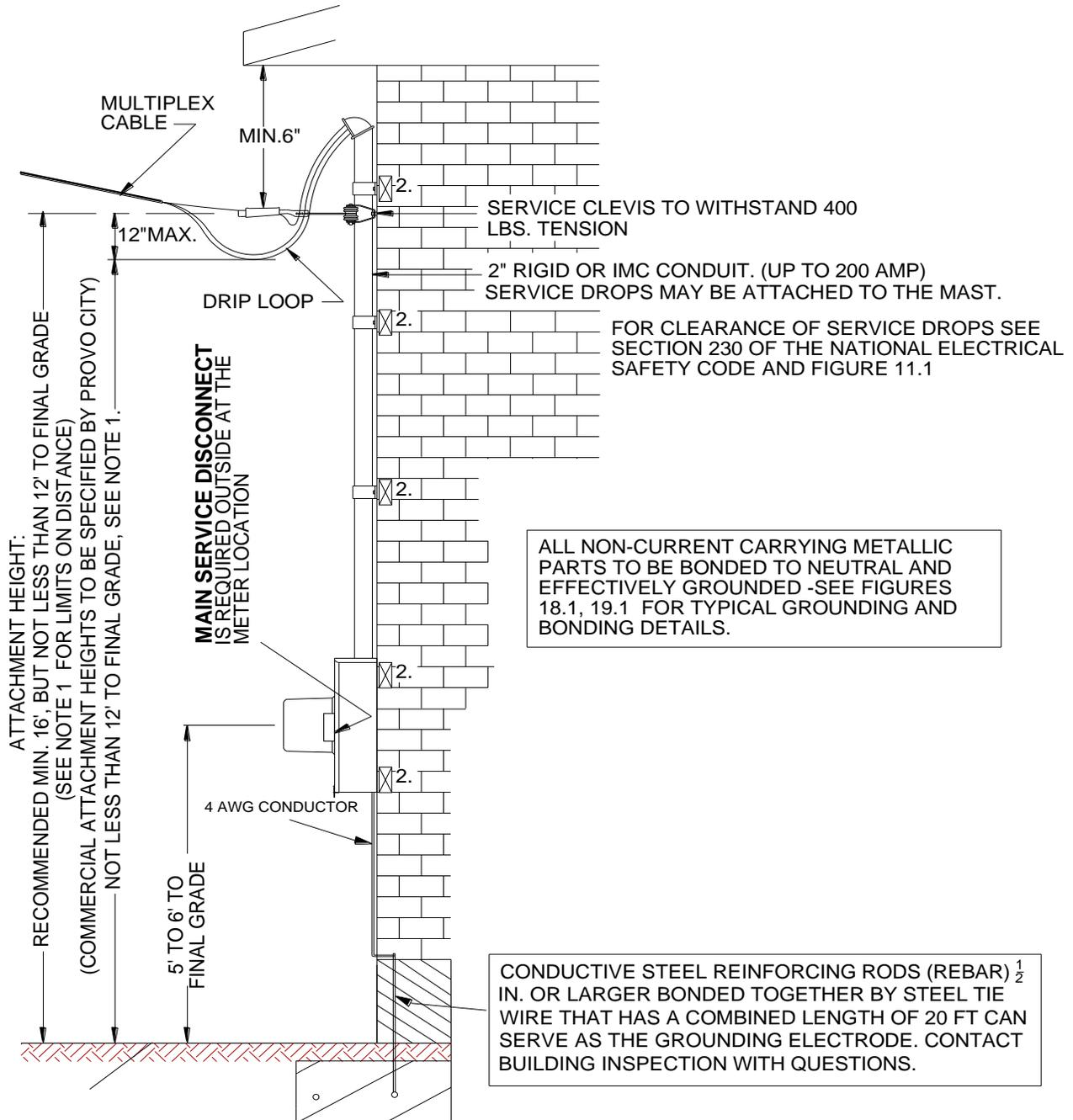
Figure 10.1 Under Eve Installation
